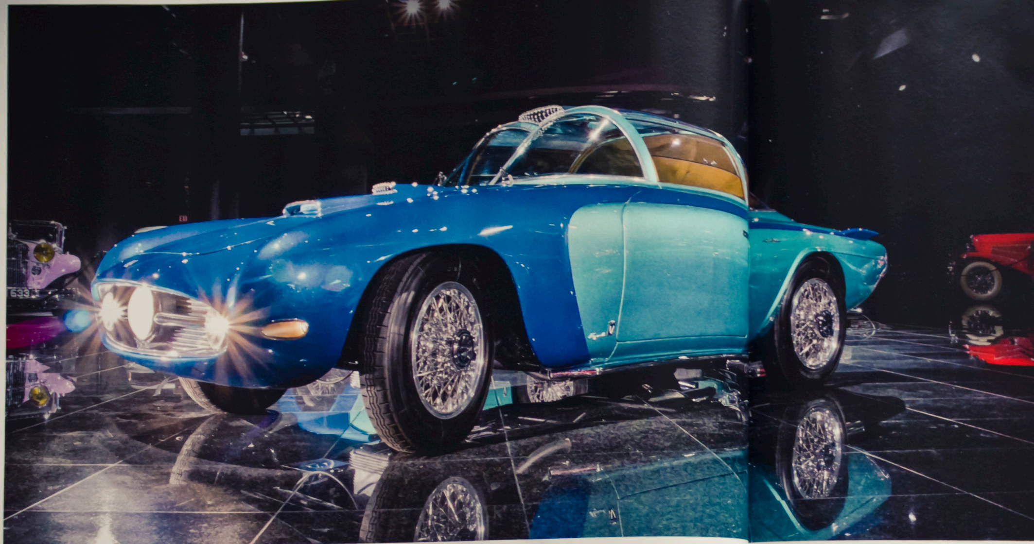
Left and below Blue Ray featured a radical fighter-jet-style canopy with a huge dome of blue-tinted Perspex, while the aluminium panels clad a tubular structure. Mechanicals came from Lancia, with Nardi upgrades.
