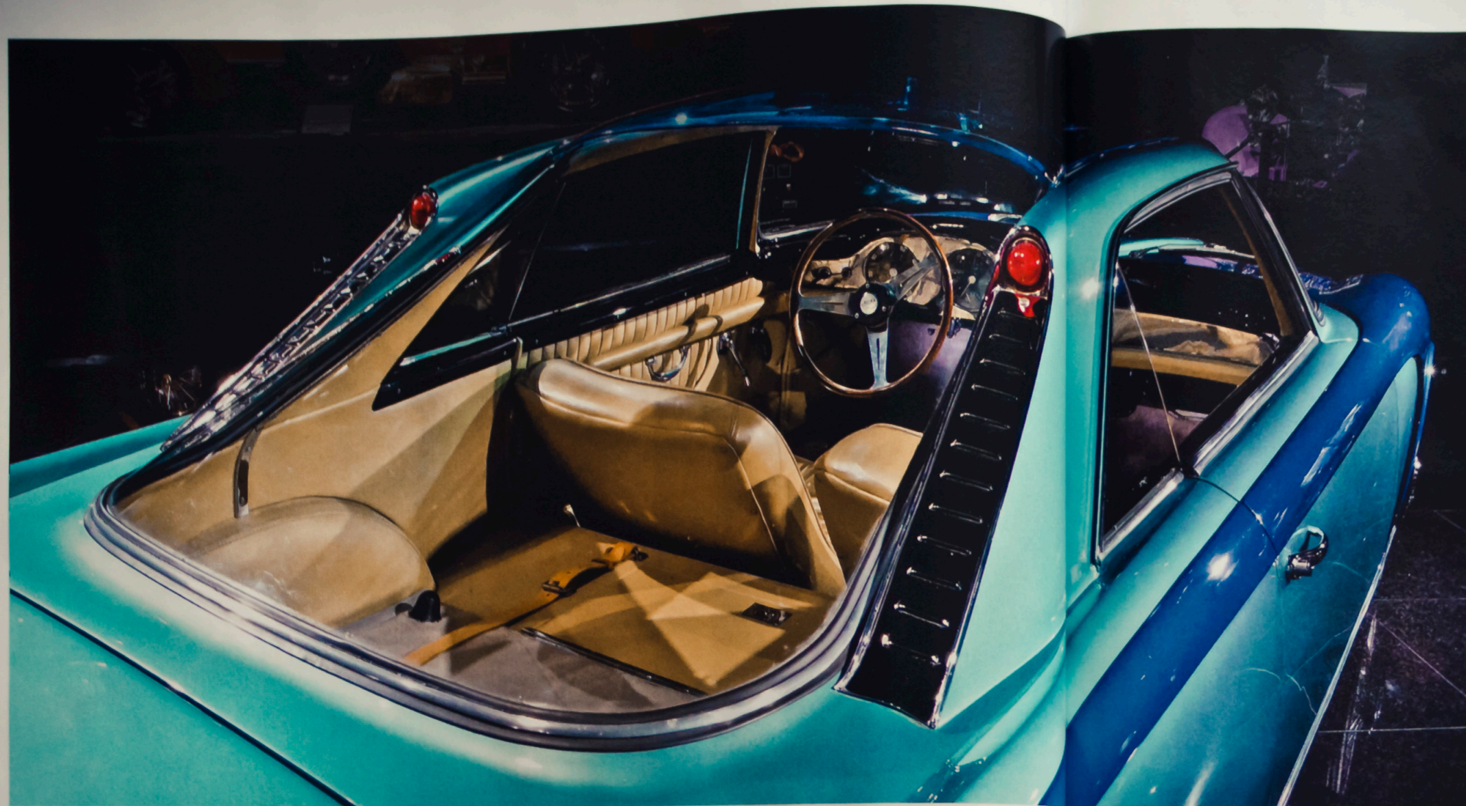
Above and right A private client ordered the Blue Ray II from Nardi, who based it around a modified Aurelia B20 chassis, clad this time in steel rather than aluminium. Aurelia mechanicals featured again, though the engine was less highly tuned than in the original.
