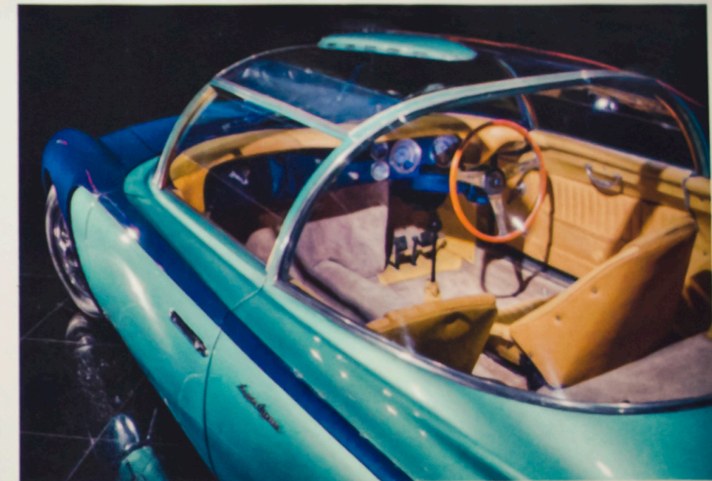
Left and below Blue Ray featured a radical fighter-jet-style canopy with a huge dome of blue-tinted Perspex, while the aluminium panels clad a tubular structure. Mechanicals came from Lancia, with Nardi upgrades.
